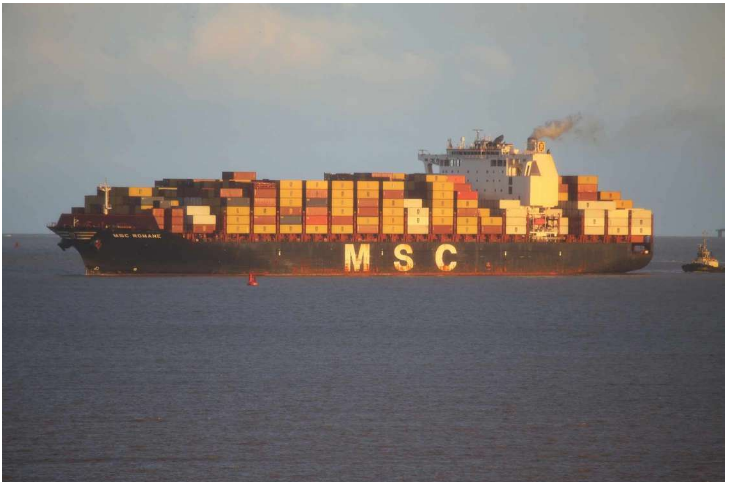
With her retrofitted exhaust scrubber much in evidence "MSC Romane" arrives from Mundra, India, Coega, South Africa and Bilbao on 30 th December. Jinhai Heavy Industries of Daishan County, China built her in 2017. (Photo by Derek Sands)
