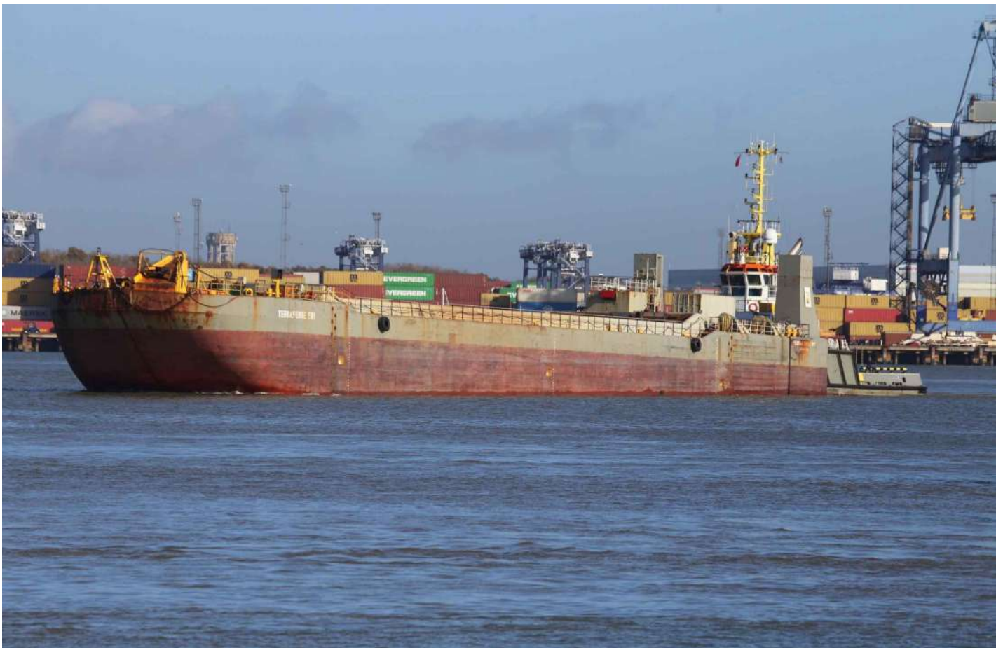
"Union Onyx" propels split hopper barge "TERRAFERRE 501" past Harwich during multiple trips in and out of the harbour. The purpose of this is so the tug master can gain a pilotage exemption certificate for their forthcoming work. The tug was built in Spain by Armon in Navia in 2008. The barge was built in 1995 by Gunderson Marine, Portland, Oregon. (Photos by Derek Sands)
