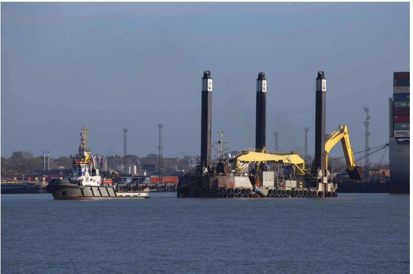
Boskalis' largest backhoe dredger "Magnor" arrives on 9 th November from Rosyth under tow from "Union Topaz" . The dredger was built in the Netherlands by Ravenstein BV in 2016. (Photo by Derek Sands)
