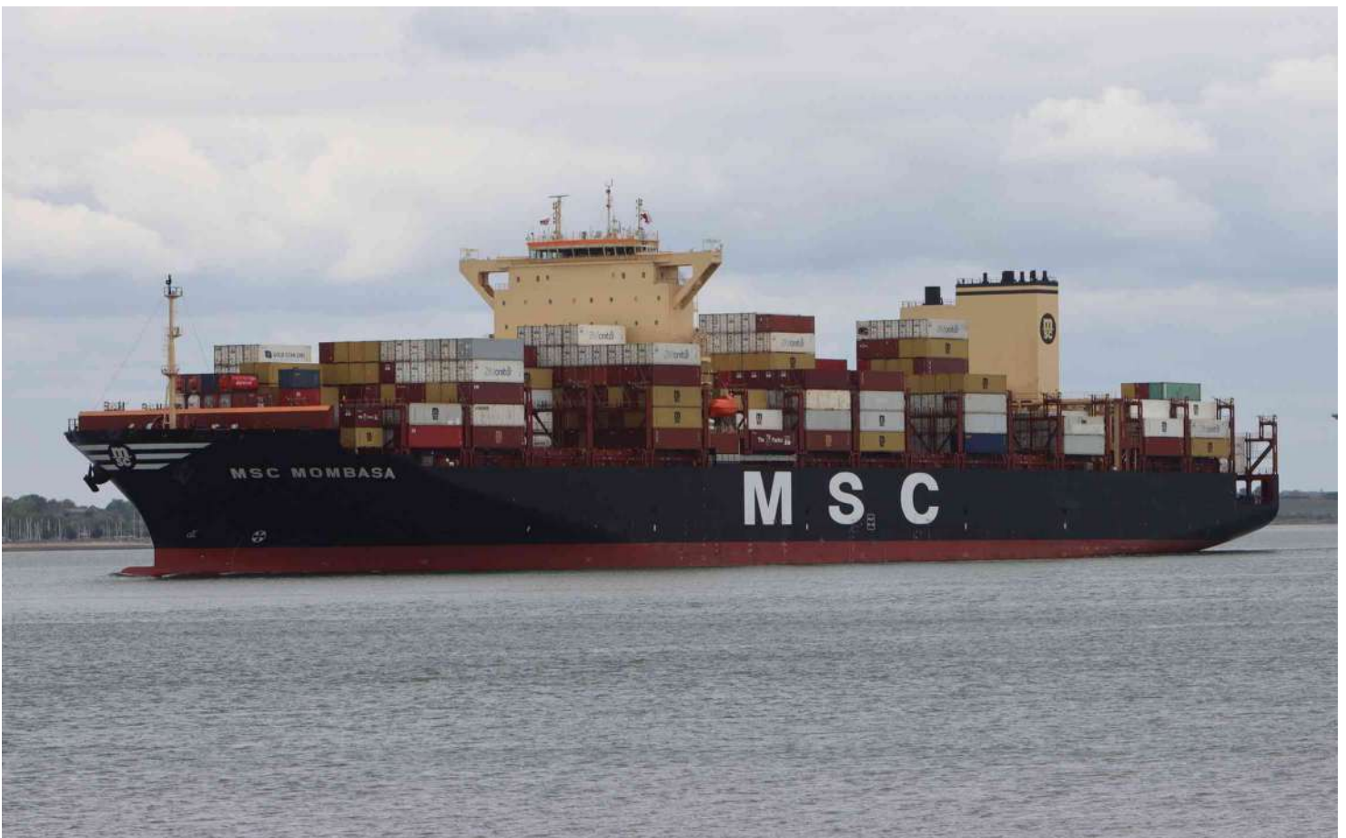
Built by Hyundai, Ulsan and fitted with an EGCS-Scrubber, “MSC Mombasa” entered service in June 2024. The 75,154 gt ship is capable of 8,030 TEU on a length of 272 metres. She arrived from Valencia on 5 th May and is seen here leaving for Rotterdam, two days later. ( Photo by David Hazell )
