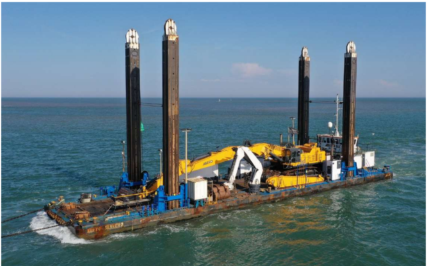
“Abeko Server 2” was built in 1997 at Hardinxveld and is registered at Beverwijk. She has a Hitachi EX1200-5 excavator. (Photo contributed)
