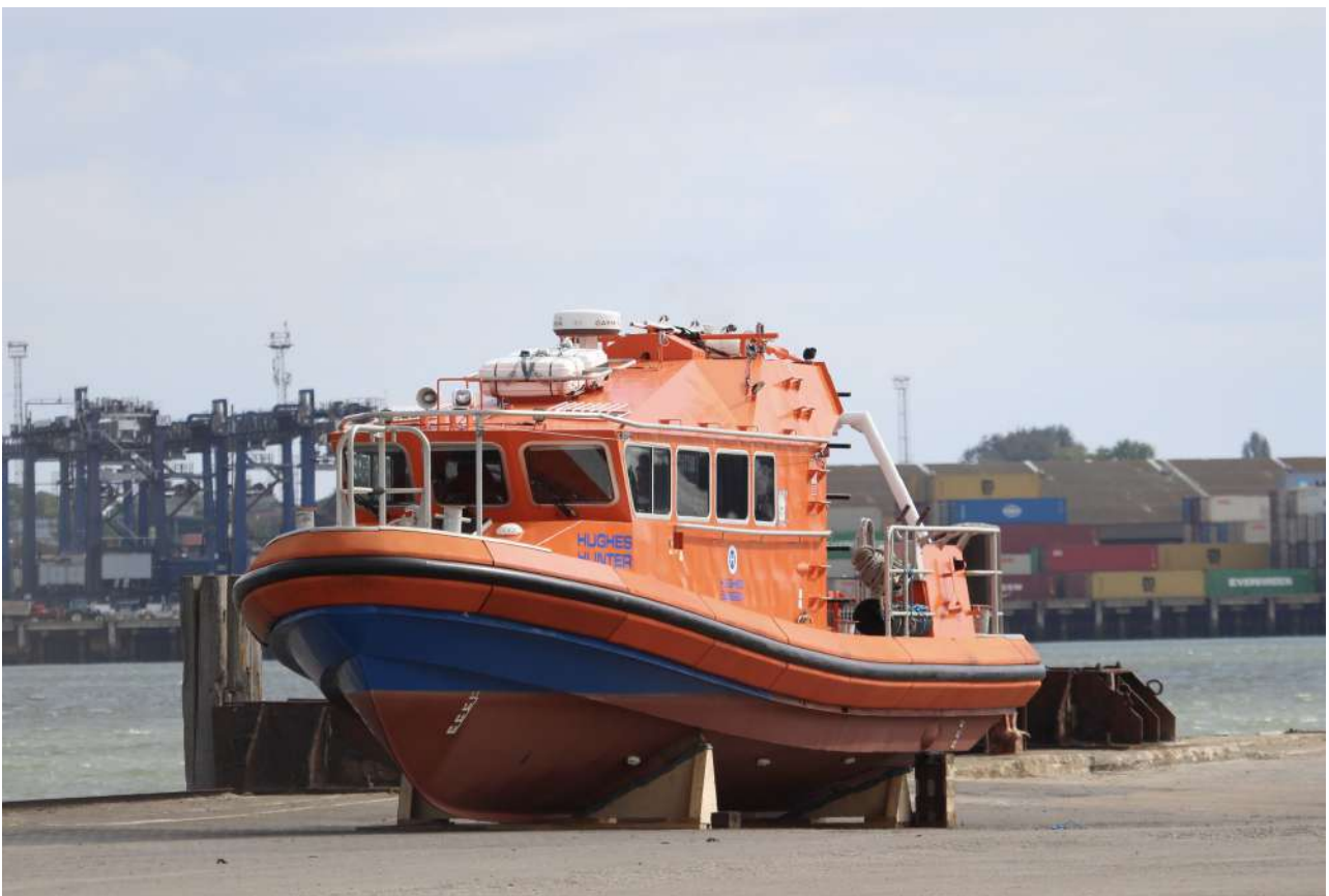
Sitting high and dry on Navyard Wharf, Harwich, “ Hughes Hunter ” has been carrying out survey work and diving ops off Harwich. She looks like she is ready for collection by road perhaps? She is powered by twin Cummings diesels driving water jets. Any more information is welcome. (Photo by Alex Dace)
