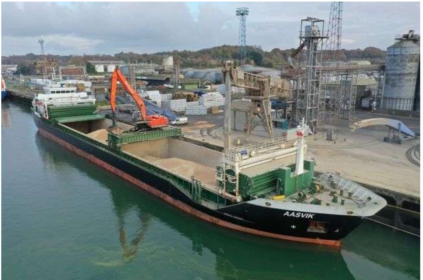
Having arrived from Port Talbot, South Wales on 30 th November, “ Aasvik ” is loading for Amsterdam at Ipswich Grain Terminal. Seen here on 1 st December she would depart later in the day for the Dutch port. Purchased by Aasen in 2017 and fitted with an excavator, she was originally “ Arklow Bridge ” and completed in May 2011 by Bodewes, Hoogezand. (Photo contributed)
