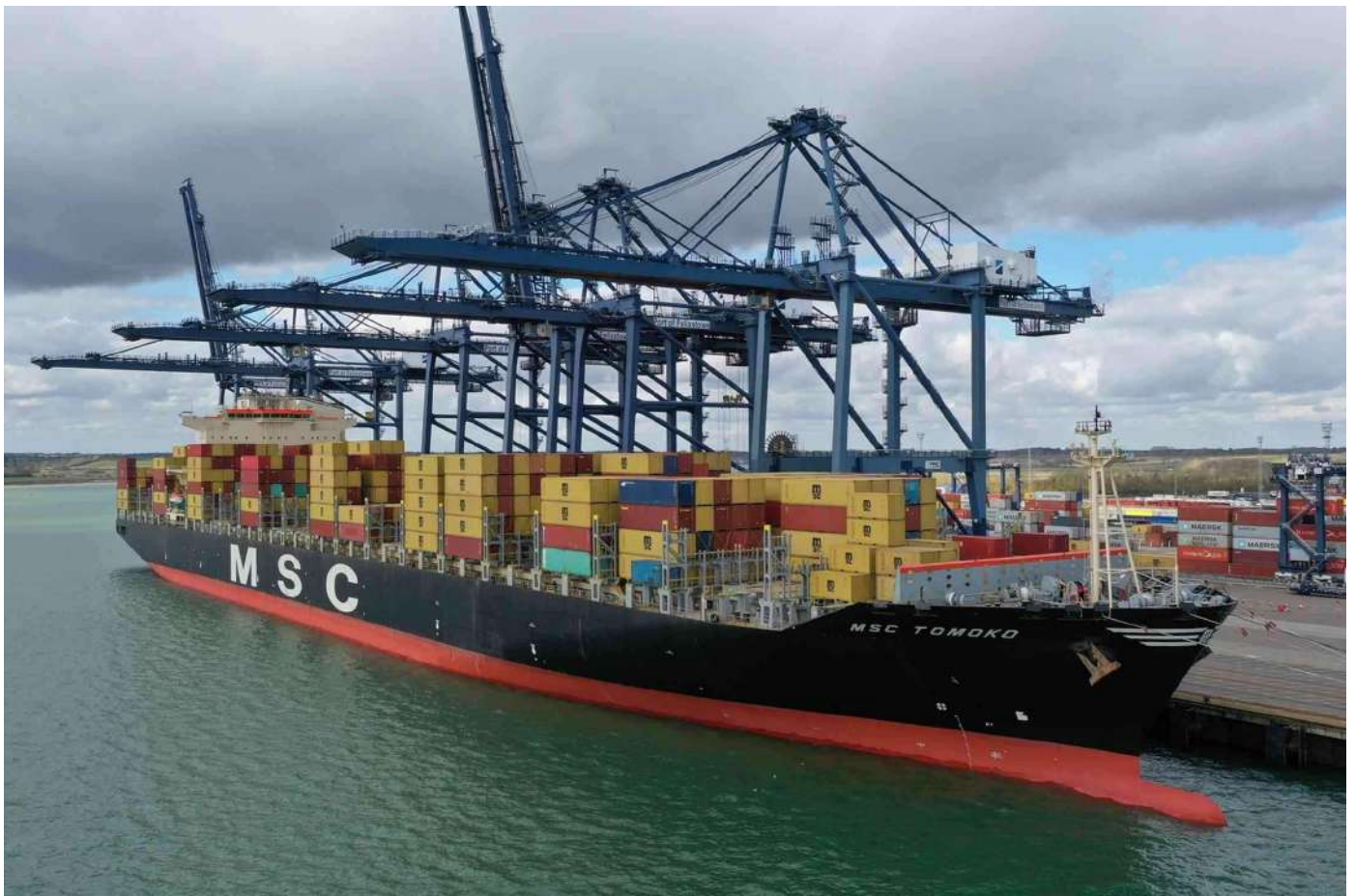
Trinity Seven berth plays host to “ MSC Tomoko ” a fairly regular caller, seen here on the 18 th March. She had arrived the previous day and would sail later on the 18 th for Hamburg. A product of South Korean yard, Daewoo, Okpo in 2006. At 332 metres long she is capable of 8,400 TEU with 700 reefer points for refrigerated containers. (Photo contributed)
