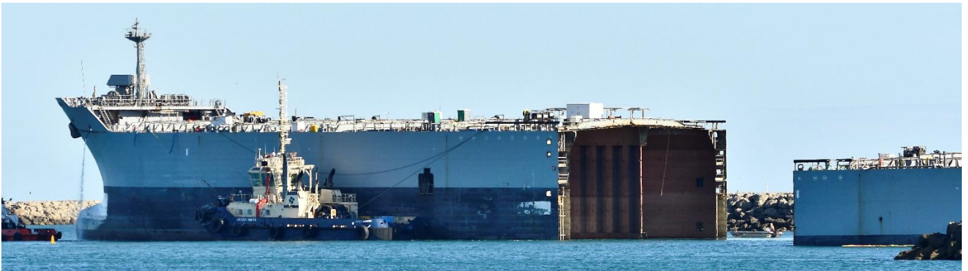
ABOVE: The now cut off & deballasted front half of SIRIUS is moved away from the still deeper stern half 28/03/2023.
