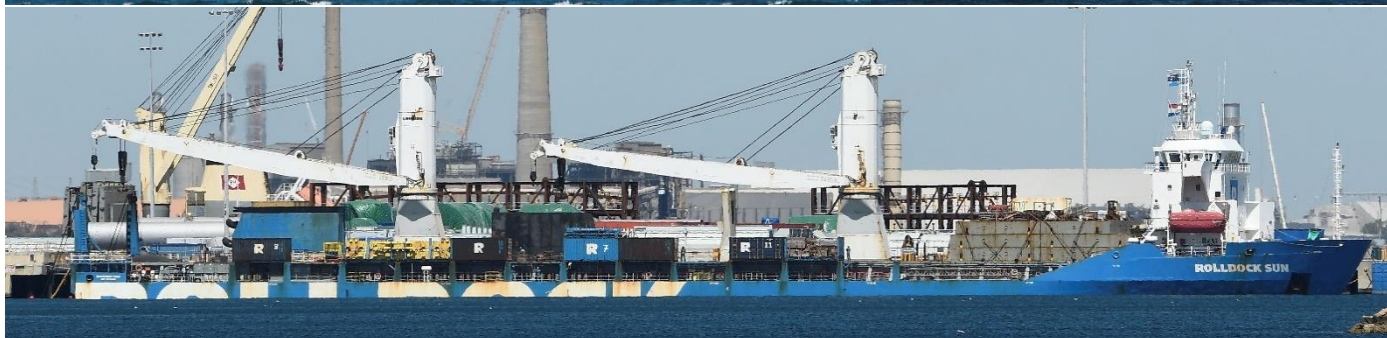
ABOVE: ROLLDOCK SUN in her fully ballasted down mode to permit OTAMA to be floated out through the stern door. BELOW: OTAMA is almost clear of the ROLLDOCK SUN's stern door and about to enter the AMC floating dock at left. In the background can be seen the former HMAS SIRIUS being scrapped at the AMC#6 berth. Both photos 29/09/2022.
