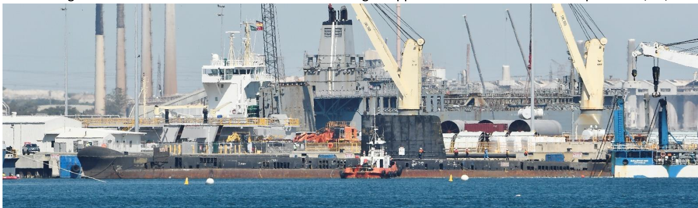
ABOVE: ROLLDOCK SUN in her fully ballasted down mode to permit OTAMA to be floated out through the stern door. BELOW: OTAMA is almost clear of the ROLLDOCK SUN's stern door and about to enter the AMC floating dock at left. In the background can be seen the former HMAS SIRIUS being scrapped at the AMC#6 berth. Both photos 29/09/2022.
