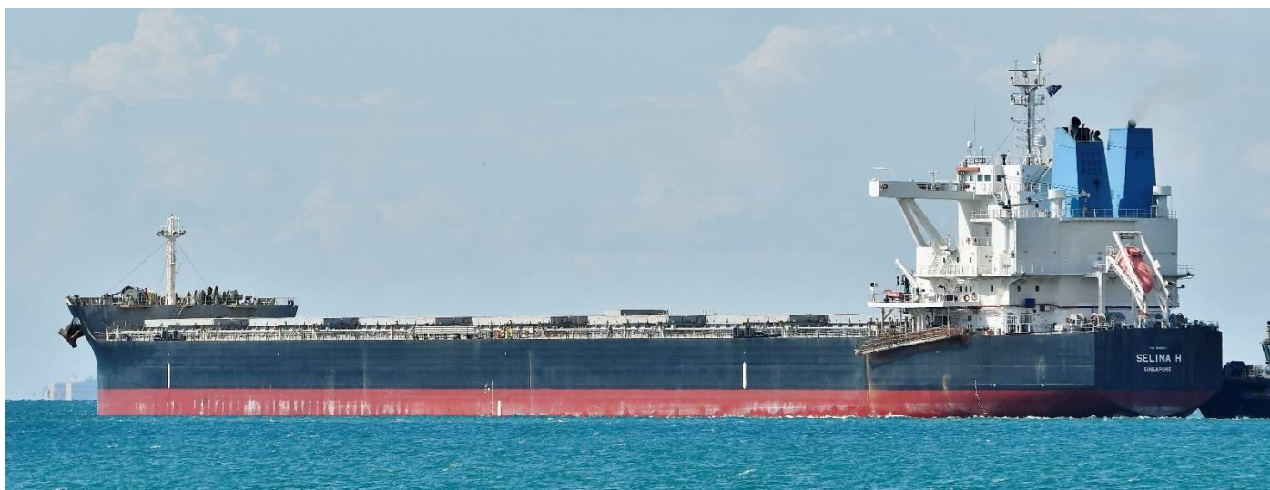
ABOVE: Another version of funnel scrubber additions with SELINA H now rendered twin funneled by the addition of the scrubber funnel mounted on the starboard side of the original funnel but somewhat designed to resemble the original. SELINA H is seen here departing Kwinana Grain Jetty 08/11/2024.
