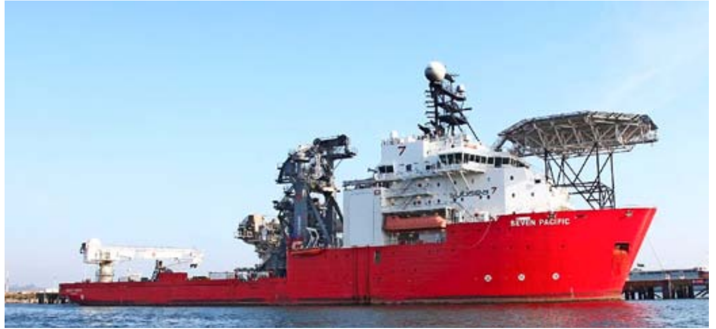
» Seven Pacific, a British-owned pipe-layer crane vessel, has been alongside Queen's Wharf waiting her turn to use number two dry dock for over a week. Owned by Subsea 7 Ltd, she was built in the Netherlands by IHC Offshore & Marine BV at Krimpen-aan-den-IJssel near Rotterdam, and registered in Douglas, Isle of Man, she entered service during November 2010. The 134m construction/flex-lay vessel is capable of operating world-wide in water depths of up to 3,000m and is equipped with a 250-ton lift crane and a 30-ton auxiliary crane. She has the capacity to load 2,500 tonnes of flexible piping on two carousels below deck. When operational she carries a crew of about 100 and has completed projects in Europe, the Mediterranean, Gulf of Mexico and most recently off West Africa in the Gulf of Guinea conducting repairs, maintenance and renewing of the pipeline from FPSO Kwame Nkrumah MV 21 (Jubilee Field)
