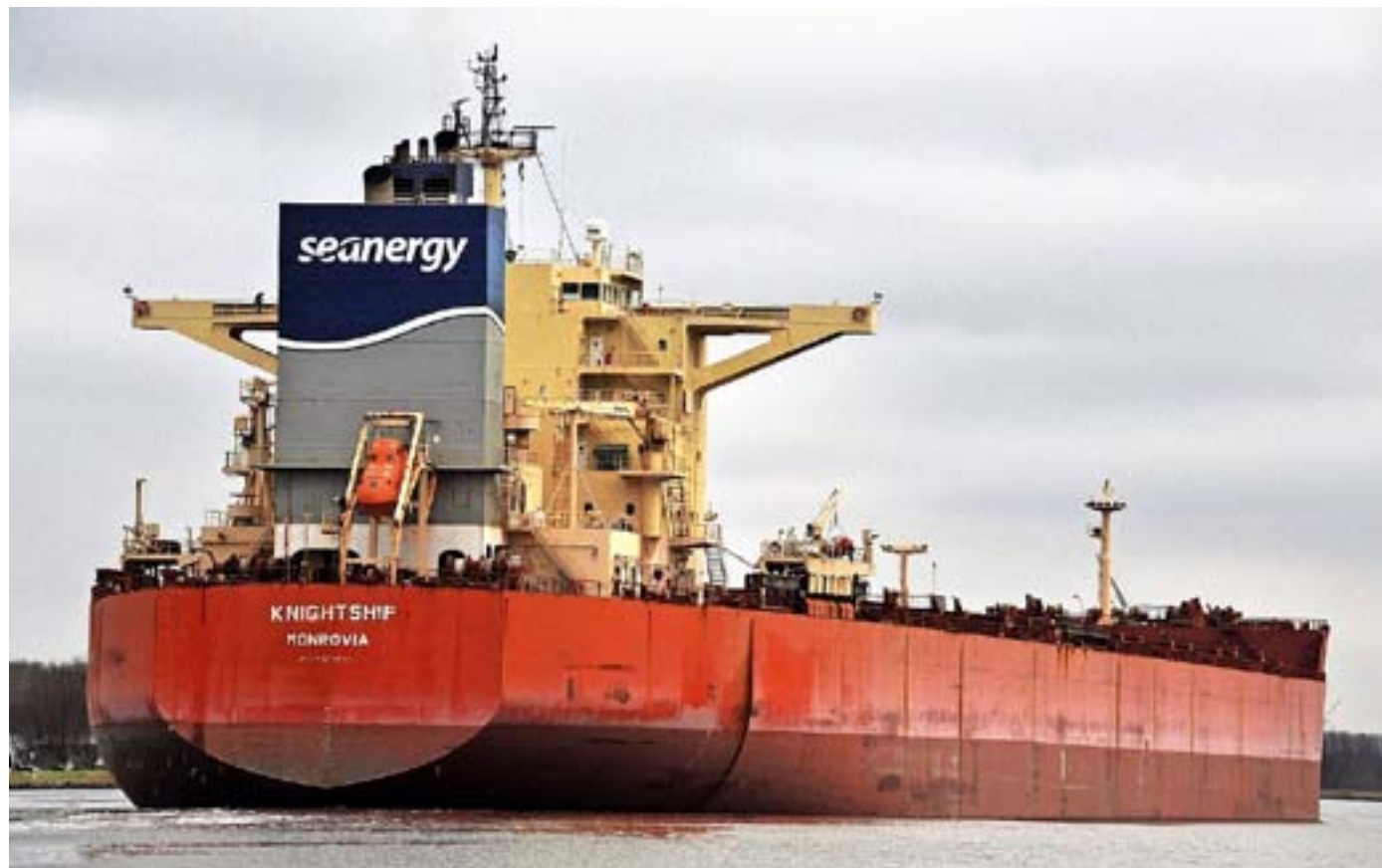
» Bulk carrier Knightship has been anchored offshore with Premiership for a few months laden with coal loaded in Queensland, Australia. She was built in South Korea for Ernst Rickmers, Hamburg, as ER Bayern, one of four sister ships. She entered service in August 2010. She has nine holds and fully laden can carry 178,980 tonnes with a draught of 18.2 metres. In December 2016 she was sold to her present owners Seanergy Maritime Holdings Corp, Athens, Greece, for a reported $20.8 million and subsequently renamed Knightship Ruud and Marcel Coster
