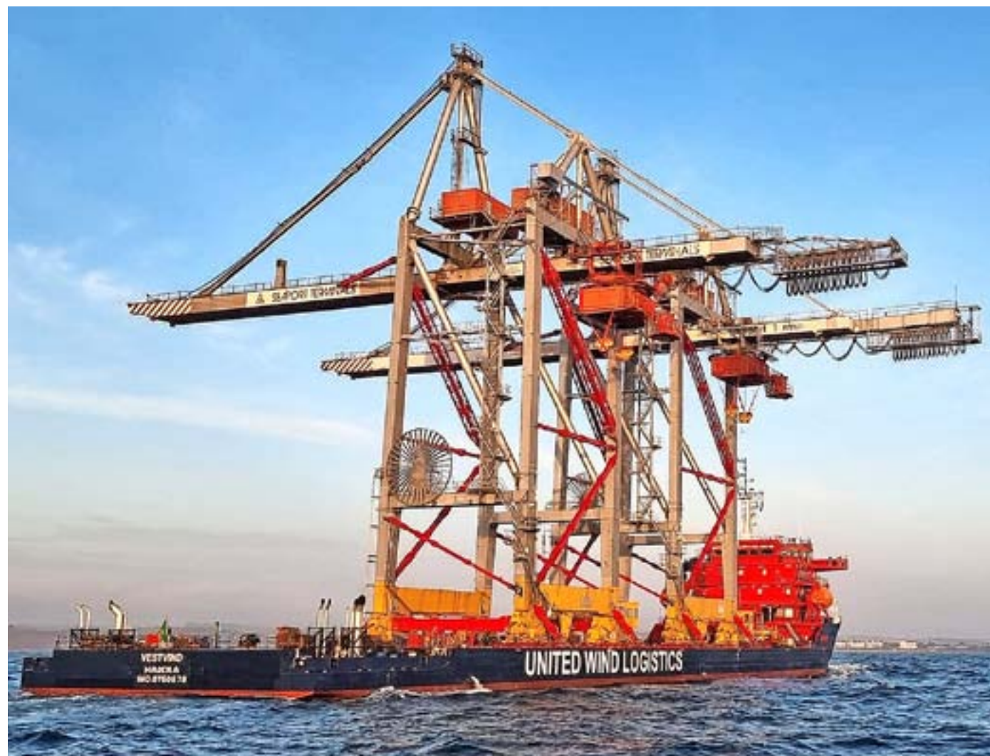
» On Sunday morning German-owned, heavy-load carrier Vestvind (7,175/16) arrived from Antwerp West and berthed alongside County Wharf. She is carrying two container cranes loaded alongside berth 1,233 at Katoen Natie Terminal in the Vrasendok area of Antwerp West. A&P have issued a port notice to mariners as the two gantry cranes extend 36m towards Port Pendennis Marina and 38m from above water level Ollie Crediton
