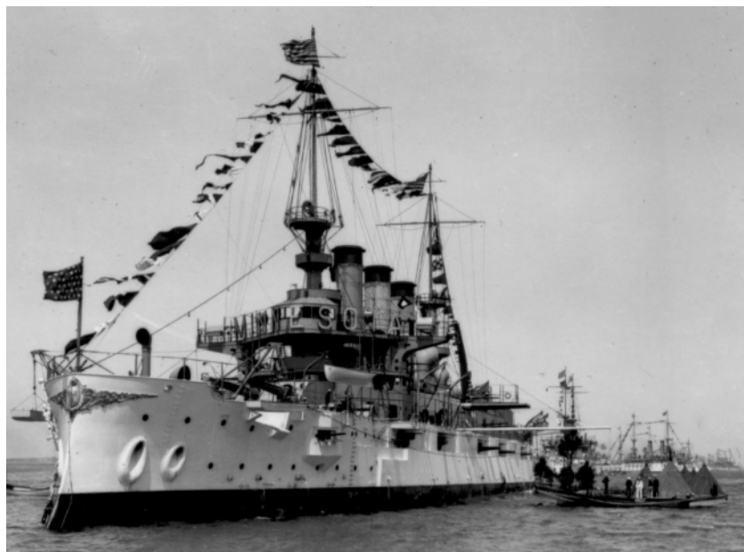
The hull casement shutters, as seen on USS Minnesota, couldn't keep water out in rough seas during the Great White Fleet's world tour, thus were eliminated in later designs. (US Navy Archives)
