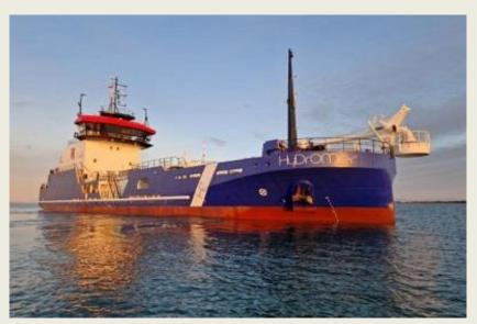
New dredger Hydromer was successfully commissioned and tested along the south-coast of France earlier this week. The 1500 m3 trailing suction hopper dredger (TSHD) was built by Chantier-Piriou from Concarneau. For this project, *HollandMT* supplied complete dredging system, including: • DN500 dragarm system, • dredge-pump, • jetwater system, • dredgepipes with bow-coupling, • hopper discharge system
