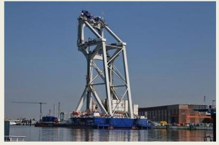
Van Oord has fitted a huge A-framed gantry extension, weighing 1,200 tonnes, to the top of its heavy-lift installation vessel **Svanen**, increasing the total height of the ship to 125 metres. The had extension been Holland constructed by Shipyard. One of the largest cranes in the world was used the installation for Mammoet Schiedam. Besides the gantry extension, the upgrade
