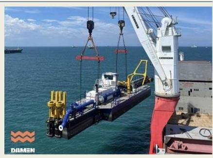
dredger is part of a complete dredging package, which includes ship transportation, training of the crew on location as well as dredge spares to facilitate maintenance duties. (Source: Dredging Today)
