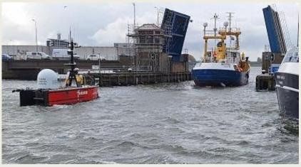
We have previously reported the use of the unmanned survey vessel Fugro Vaquita. Last week, photographer Wim Albers captured the 12-meterlong vessel as it neatly followed SeaMar's mother ship **Alcedo**. The **Fugro Vaquita** was operated remotely by operator standing at the back of the deck of the Alcedo. Both vessels have been operating at
