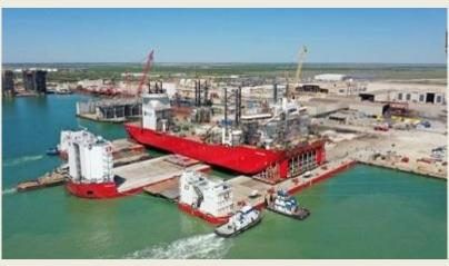
three-barge simultaneous ballasting operation. The WTIV launch is also notable for setting the record for the world's largest load out totaling 26,000 tons including the world's largest SPMT assembly of 880 axles. Congratulations to all involved in this operation, and we wish Dominion and the crew of the Charybdis good luck with their new vessel! We thank Fagioli for being a valued client of BOA. (*PR*)
