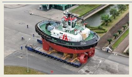
On 12th April Damen Shipyards Group launched the second of its fully electric RSD-E Tugs 2513 at Damen Song Cam Shipyard. The tug is being built for the Port of Antwerp-Bruges, together with five conventional RSD Tugs 2513. When delivered later this year, it will be the first fully electric tug to operate in European waters. The port was one of the first to operate a
